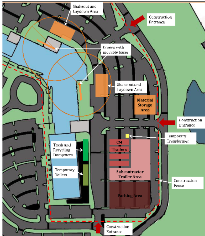
Figure 5: Site layout planning for the superstructure phase
